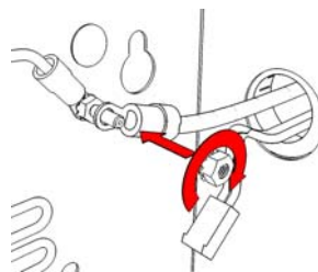
Figure 14. Auxiliary pump box ground wire connection
